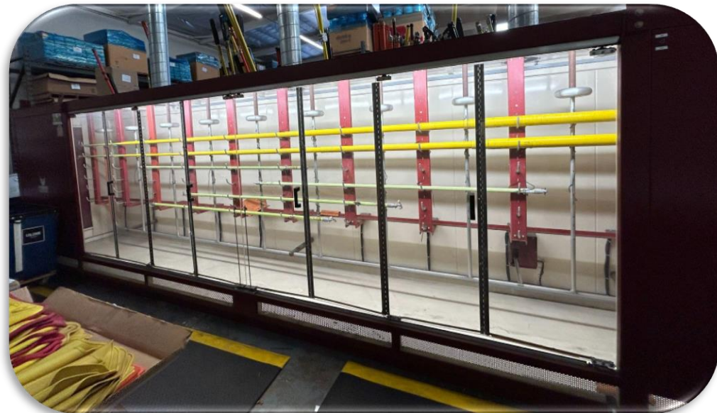
Figure 2 - Hotstick Dielectric Testing
